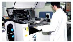
In a project of direct innovation in Productive Processes for Electronic Products, the CPC staff in partnership with the CERTI Amazônia Institute conducted the complete development of productive processes for a new circuit board for the POSITIVO Informática company. For the different lots and products developed, activities were conducted ranging from analyses of suitablity of the design to analyses of manufacturing (DFx and DFm), development of documents to provide guidance for the
